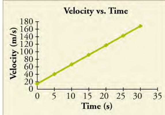
True or False:—The image shows a velocity vs. time graph for a jet car. If you take the slope at any point on the graph, the jet car's acceleration will be  $5.0 \text{ m/s}^2$ .
