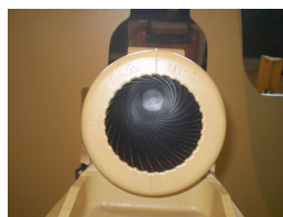
Figure 6.E. 5: The image shows a view down the barrel of a cannon, emphasizing its rifling. Rifling in the barrel of a canon causes the projectile to spin just as is the case for rifles (hence the name for the grooves in the barrel). (credit: Elsie esq., Flickr)
