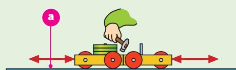
Spring is released by hitting with a hammer
