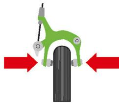
**When you pull the brakes** on a bike, the force of friction between the brakes and wheel does negative work. Friction transfers energy from the bike’s kinetic energy store to thermal energy, making the bike slow down.
