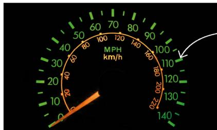
This car speedometer shows speed in both miles per hour (green) and kilometers per hour (orange).
